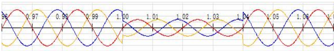
Figure 4.2.2.3.9.2 Waveform Screenshot of Voltage dip
