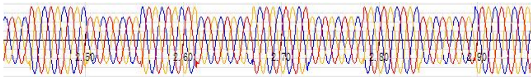
Figure 4.2.2.3.8.1 Waveform Screenshot of Voltage Flicker
