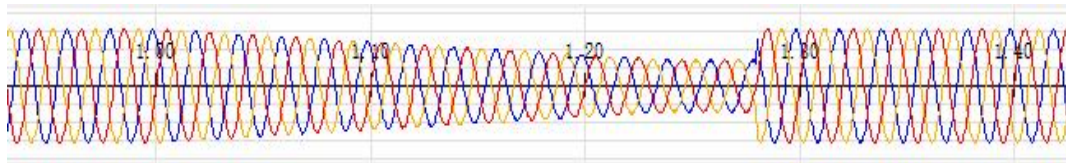
Figure 4.2.5 Waveform Screenshot of Rapid Voltage Change
